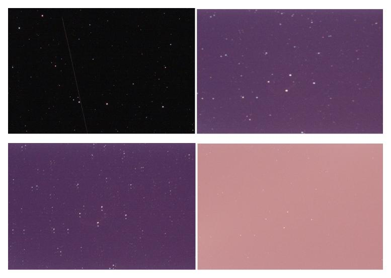
You might also want to click on "Compute offsets" and then sort by dX, dY and Angle. This is in particular true if your are working from a balcony, where vibrations are more prone to happen. The vibrated frames will be more easily detected by sorting by those, as well as by #Stars.
