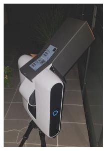
After about 30 to 45 minutes of capture, place a dark object over Stellina's arm to block all light from reaching its sensor. The cardboard box of Stellina's Gitzo tripod fits perfectly (see picture). Leave it like that for 5 to 10 minutes. You can then continue with your capture normally. The FITS collected during that period will be your darks.
